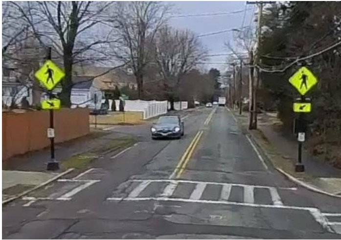
Figure 44. Rectangular Rapid Flashing Beacons (RRFBs)
